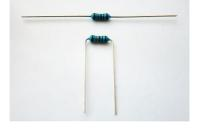
Bend the resistor leads as close to the body as possible, fit them in the footprint and once soldered cut the excess of lead as short as possible to avoid short circuits.
