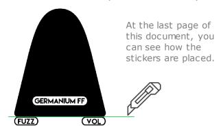
Place the 2 plastic insulators (one need to be cut following the stencil) using double side tape, they will protect the electronics:
