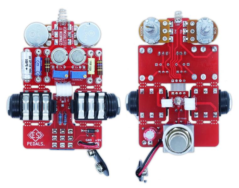
Note: The LED is still not soldered, once inside the enclosure you can adjust the perfect length for the leads and solder it.
