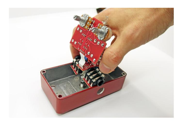
When all is in place, you can finally fit the washers & nuts and solder the red LED.
